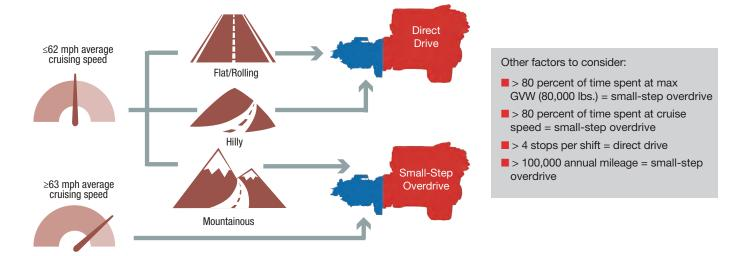
Use this guick reference guide to determine which SmartAdvantage Powertrain is right for you.
